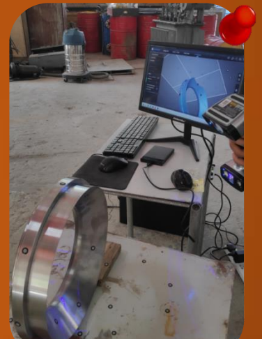
3D scanning of Pelton turbines of Rahughat Hydropower Plant (Cascade I and II) conducted by Nyano Care Pvt. Ltd. in partnership with TTL on July 26
