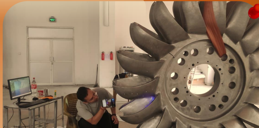
3D scanning of Pelton turbines of Rahughat Hydropower Plant (Cascade I and II) conducted by Nyano Care Pvt. Ltd. in partnership with TTL on July 26
