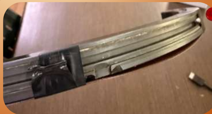
Reverse engineering of a shaft seal of a Francis turbine of Molung hydropower plant
