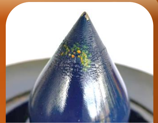
Erosion test performed by Mr. Prithvi Gurung on a Pelton injector (Mid opening of needle)
