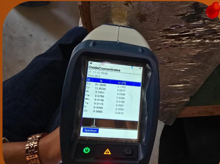
Material constituents studied for the broken piece of Kaligandaki HPP through a XRF analyzer
