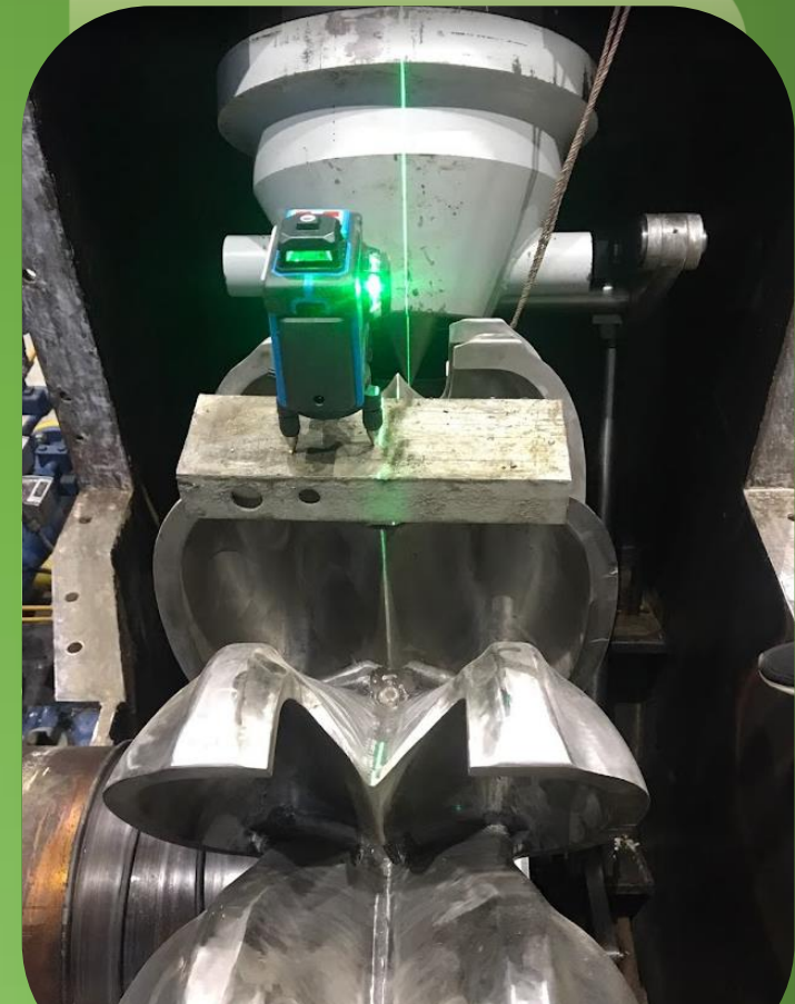
Misalignment test conducted on the turbines of Ghar Khola HPP
