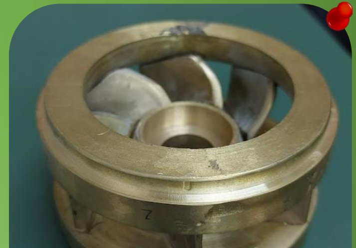
Sand casted Francis runner developed as HRCHR co-operation between WHU and KU for Master's study of Mr. Ravi Poudel
