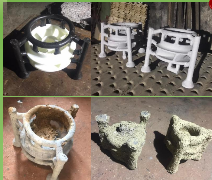
Progresses of Lost PLA casting of the turbine in process from NTIC project
