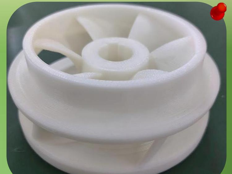
3D printed impeller designed at TTL, currently in the fabrication process
