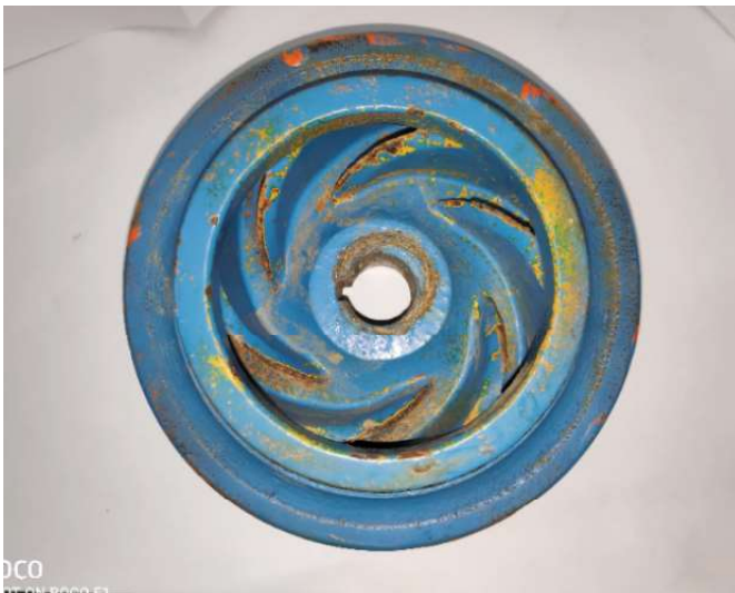
Fig. 1 Erosion Pattern in pump impeller
