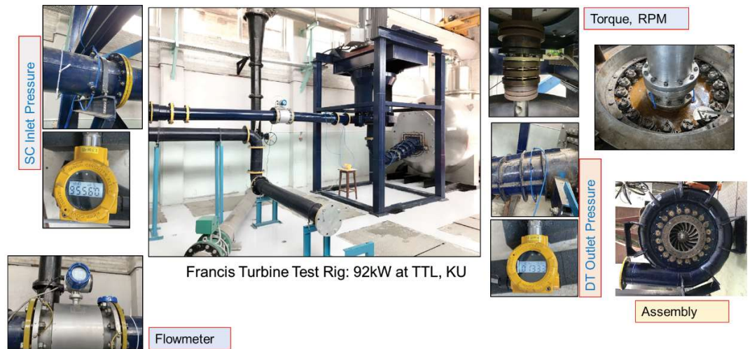
Fig. 1 Experimental set up for 92 kW Francis turbine
