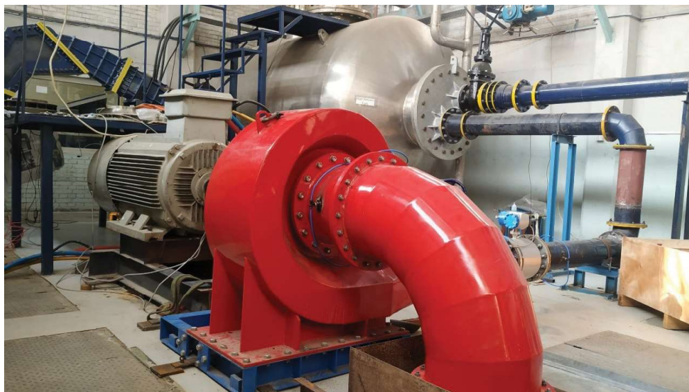
Fig. 1 Laboratory testing of Francis turbine of Chauri Khola II MHP
