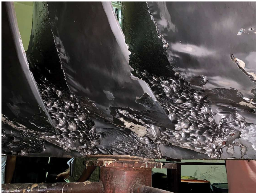
Fig. 2 Sediment erosion of runner at Kaligandaki hydropower plant
