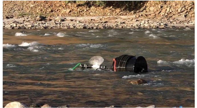
River water pump (coil pump) tested during the project TTL-IRDP. The project was funded by KOICA under KU IRDP program for the period of 2020-2021.
