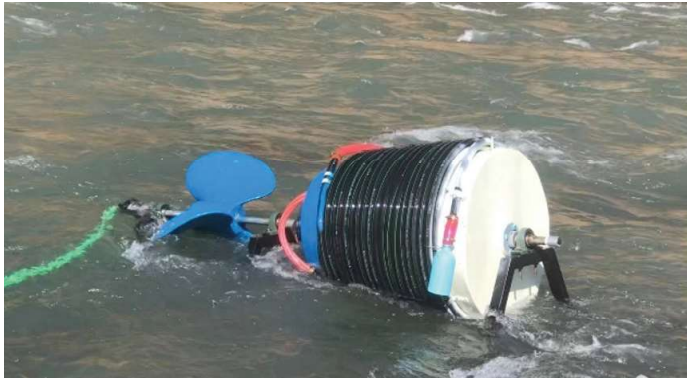
River water pump (coil pump) tested during the project TTL-IRDP. The project was funded by KOICA under KU IRDP program for the period of 2020-2021.
