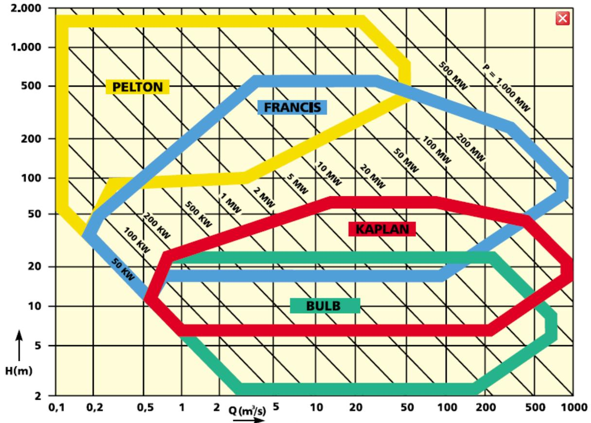
**Figure 1** Turbine Selection Chart based on Head and flow rate [2]
