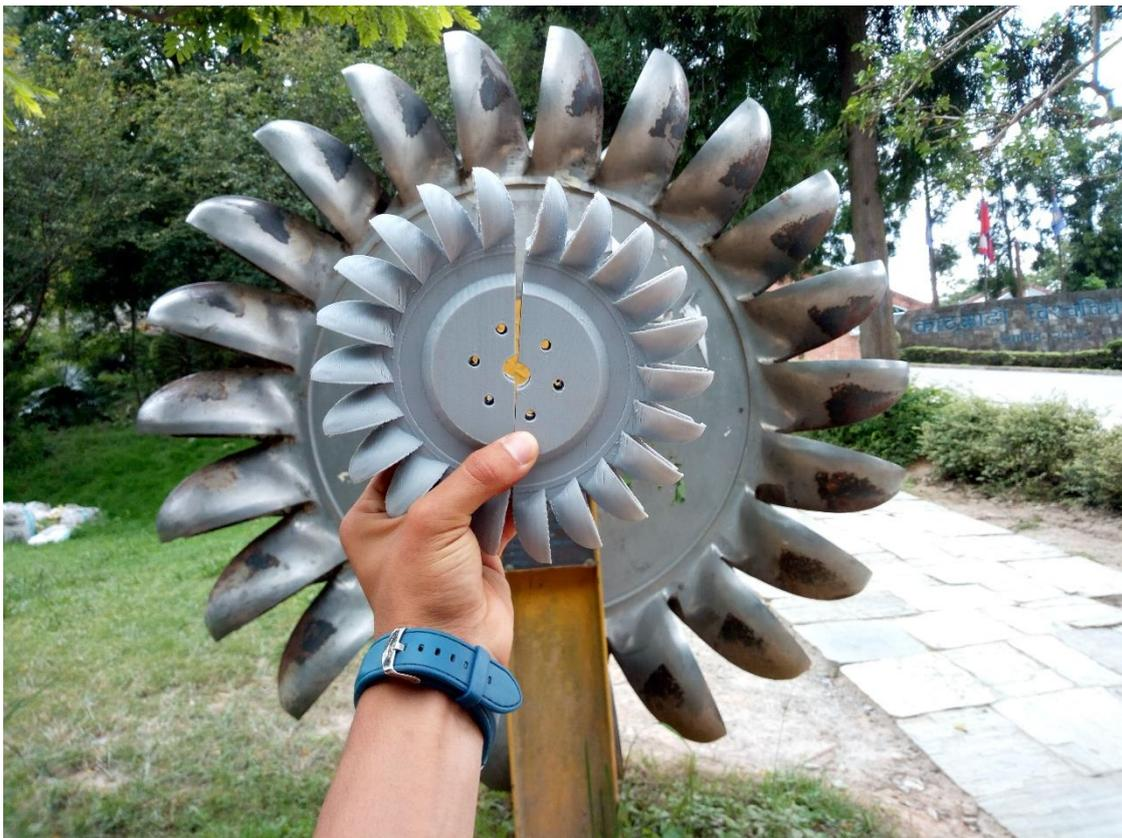
**Figure 1.2** Casted and Rapid prototyped model of Pelton Runner
