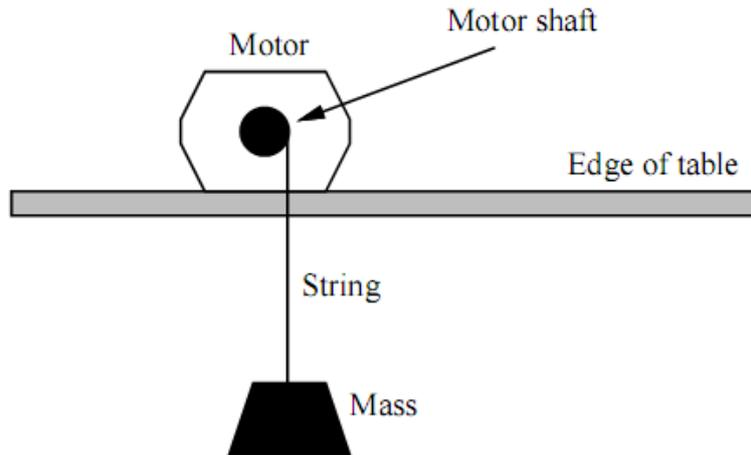
**Figure 4.4** Torque measurement method
